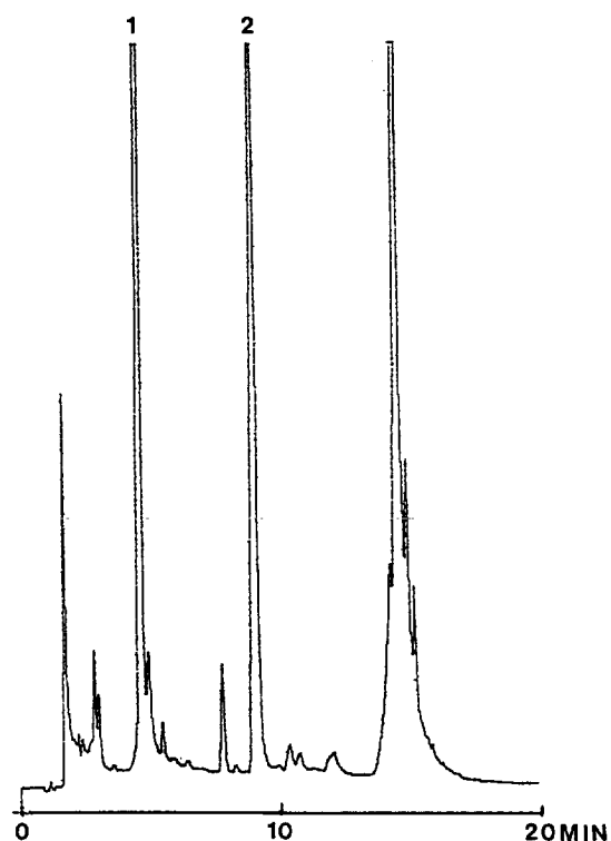
Fig. 8. HPLC chromatogram of beer sample. Flow-rate, 0.7 ml/min (Jasco pump). Mobile phase: A=acetonitrile, B=distilled water. Gradient: A=10% for 10 min, subsequently from 10–100% in 2 min. Peaks 1 and 2 were collected.
